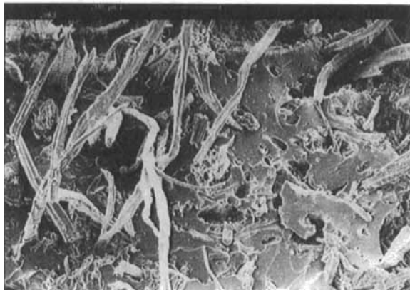
FIGURE 4 SEM micrograph of the rubberwood fibre filled natural rubber composites after tensile fracture at various filler loadings (a) 0 phr (control composite) (b) 10 phr (c) 20 phr (d) 30 phr (e) 50 phr at magnification X 150.
